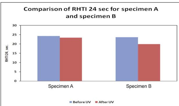
Fig. 8. Comparison of Radiant Heat Transmission Index RHTI 24 sec
